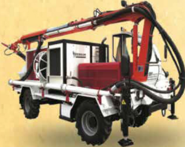
ROBO 4X4-34 EK SHOTCRETE
