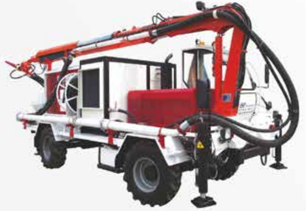
ROBO-25 4X4 EK SHOTCRETE
