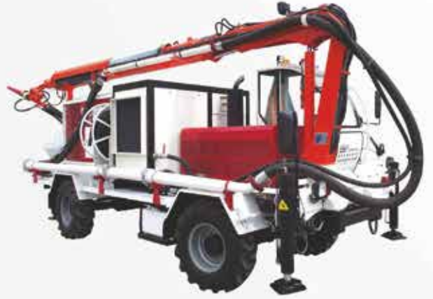
ROBO-25 4X4 EK SHOTCRETE
