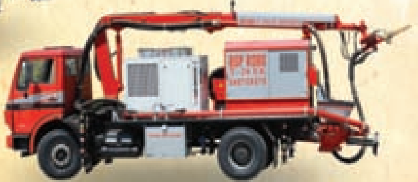
ROBO T-28 EK SHOTCRETE
